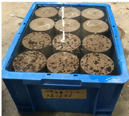
Fig. 2 Immersion of specimens into impregnation solution.
